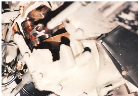
Hole in Crankcase and broken rod
